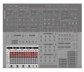
The arpeggiator has a built in sequencer for making rhythmic patterns. Each step of the pattern sequencer offers on/off, Tie, Slide, Tune, Velocity settings and also, Free modulation settings. To turn on the arpeggiator select the 'Play Mode section' of Predator-RE. To see the arpeggiator controls click on the > Arp button if the 'Free modulation section' is open.
