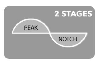
**STAGE** number determines the number of notches and peaks in 360° phase-shifting. Peak or Notch have 180° shifting.
