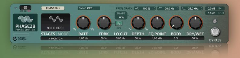
Introducing **PHASE28**, a new phase shifter effect. The Stages selector gives you control of how many stages from 2 to 8. Use 4 for a classic 4-stage phaser, or 2 stages for subtle shimmer effects. You can increase the stages to 6 or 8 stages for new creative experiments.
