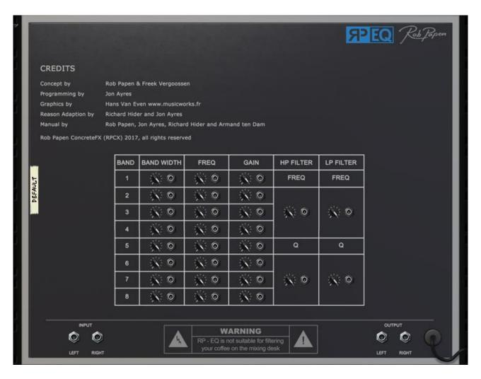
The back screen of RP-EQ shows the Input / Output audio connections and also CV input to each band's frequency, bandwidth & gain, also the Low-pass / High-pass filter frequency and Q(resonance).
