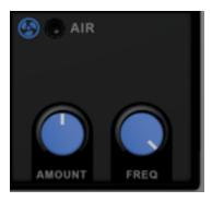
RP-EQ has an additional EQ band, which boosts the very high frequencies at a wide band, to give the sound more 'air'.
