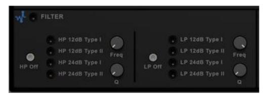
After going through the EQ, the signal passes through a high pass & low pass filter. Most obvious use of this filter is to use the HP filter with a setting of 75 kHz like many classic mixers have. We added 12dB and 24dB, but also different sound colours. The LP filter is not very common on a mixer, but can still be handy if you simply want to roll off the high end on a certain track in your music piece. We also have two types of colour filters.
