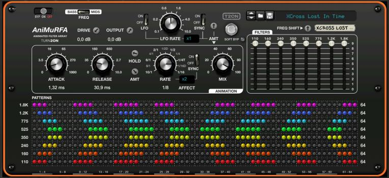
A device based on the well-known hardware pedal in the synthesizer and guitar worlds as world-class effects. This is an 8-band resonance filters array and "Animation" generator of envelope sequences. 8-bands filter array is available in selectable Bass or Mid-frequency response (with own bands frequency range). Animated envelopes modulate the levels of the 8-band filter array.
