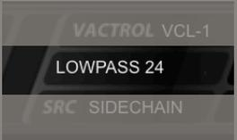
When the device is running in either BOTH or FILTER modes the incoming sound is affected by the filter. In VCA mode the filter is disabled. The filter is set by default to LowPass 12dB/oct, which emulates an LPG. xLPG offers 9 internal filter types which add new possibilities for creating not only LowPass Gate effects, but also modes such as BandPass Gate, Comb Gate, etc.
