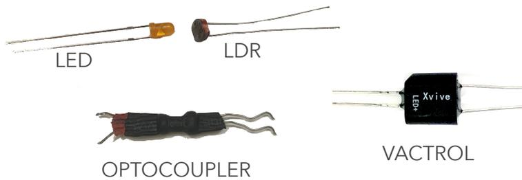
A Vactrol is a resistive opto-isolator, or photoresistive opto-isolator. The simplest form of Vactrol is an analogue optoisolator (Optocoupler). Optocouplers are comprised of a light dependent sensor (LDR) and a light source (LED), housed within a light-isolated casing. Increasing the LED brightness causes a decrease in the LDR resistance.
