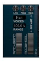
Pitch Bend: This standard wheel is used for pitch notes. Range of this wheel you can set with Pitch Range knob (max to -1/+1 octave).
