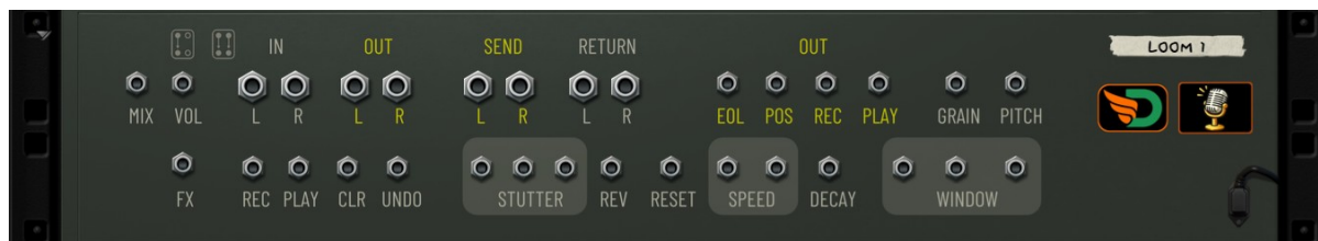
LooLoo Mini back panel — audio I/O, FX send/return, and the CV system.
