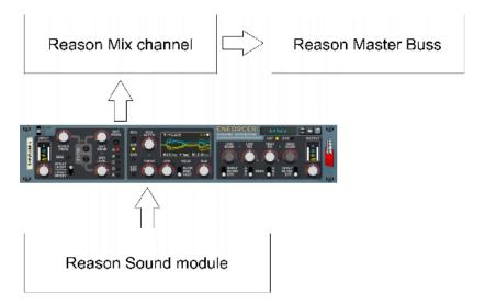
In the above setup, Enforcer would technically be an insert effect. We say technically because the signal flow comes in and passes out again. However, Enforcer has the addition of a dry level control, as well as having a saturated signal mixed with the dry, making this a parallel processing device (much alike a send-and-return style of unit).
