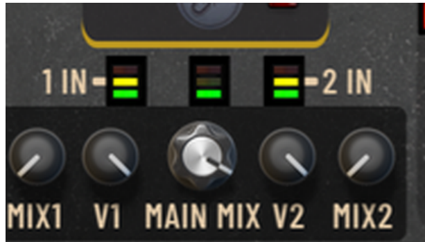
Central input/mix section: per-track levels and the MAIN MIX master.
