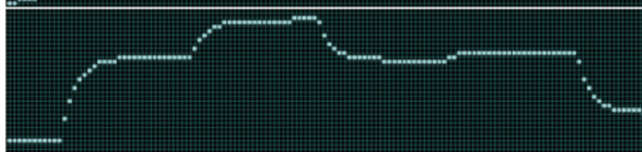
Random waveform with 50% logarithmic Lag Up and 50% logarithmic Lag Down applied. Both rising and falling edges are smoothed with a curve; in this scenario the device acts like SubTractor's Smooth Random
