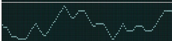
Random waveform with 50% linear Lag Up and 50% linear Lag Down applied. Both rising and falling edges are smoothed creating a random triangular waveform
