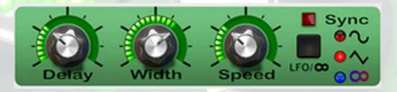
**Delay**: Up to 6.3 ms of delay with respect to the dry signal
