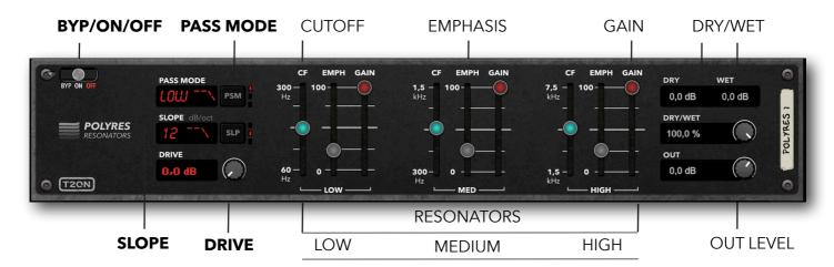
PASS MODE Original hardaware resonator section in early polysynth has a three-position PASS MODE switch that selects filter mode for all three resonator bands (Low, Medium, High).
