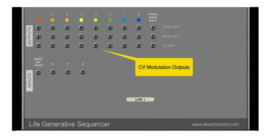
Each cell color has dedicated controls in the front of the device for setting the base CV value and any CV variation. There is a switch in the upper right corner of the Output section which allows access to the CV controls.
