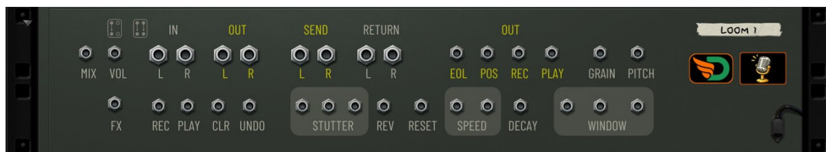
The LooLoo Mini back panel — audio I/O, the FX send/return pair, and the CV system.
