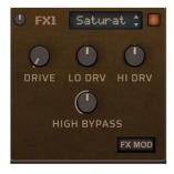
**Drive**: increases the input level resulting in more saturation and more level
