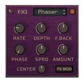
Rate: modulation rate in Hz
