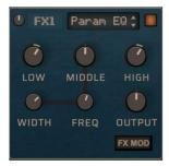
Low Gain: boosts or cuts low frequencies, low shelf is at 160 Hz
