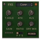
Threshold: audio level above which compression is applied
