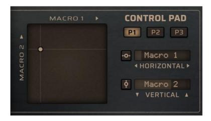
You can define three control pads (controller pairs), and easily switch among them with **P1**, **P2**, **P3** radio buttons.
