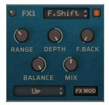
**Range**: frequency shift in Hertz. Low values result in barber's pole phasing when Mix is set to 50%.
