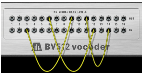
Using the Transfer Curve function in BV-X is similar to cross-connecting band levels in the BV512 Digital Vocoder.
