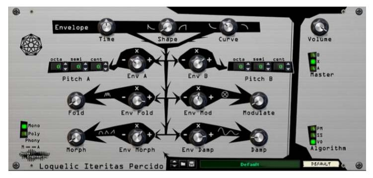
**Envelope Sends -** six attenuverters that route envelope to pitches and parameters. Positioned at 12:00, the envelope is off and does not route to a parameter. Fully CCW results in an inverted envelope send. Fully CW yields full positive send.
