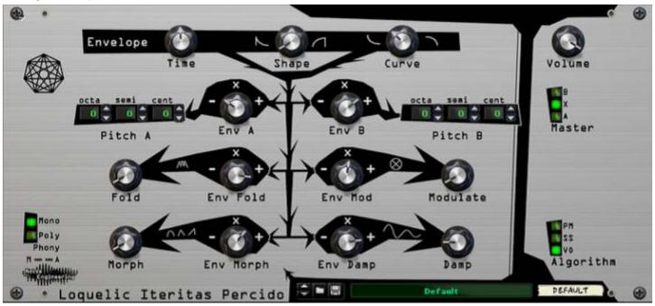
**Pitch A/B** - The pitch selector adjusts the pitch of each oscillator. Define octave, semitone, and cent.
