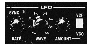
The Global LFO (Low-Frequency Oscillator) can be used as a mod source for the PWM (amount set at each OSC) for modulating VCF (Filter cutoff frequency) or VCO (oscillator pitch).
