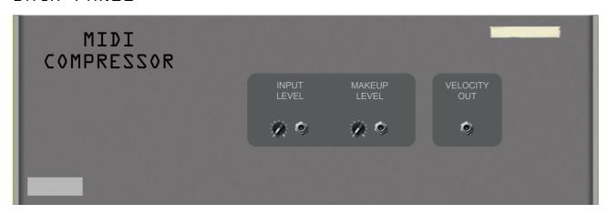
The back panel contains CV inputs for controlling the **INPUT LEVEL** and **MAKEUP LEVEL**. When a cable is connected to one of these sockets, the CV signal is added to the current setting of the corresponding knob. Note that you can subtract from the current knob value by using a negative (bipolar) CV signal.
