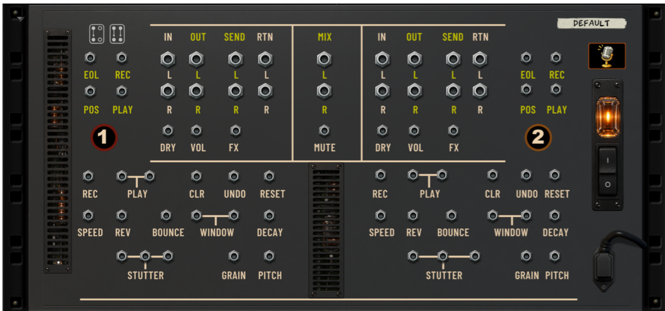
Back panel: per-track audio jacks and CV columns, the central Mix bus and mute gate, per-track CV outputs (EOL / POS / REC / PLAY), and the parameter CV inputs.
