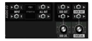
**ODD/EVEN Outputs**: Routes Even and Odd frequency bands to separate stereo outputs for advanced mixing and effects processing.
