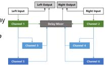
The **Delay Time**, **Delay Type** selector text and the Link Lamps are split between green for the cross stereo on Delay Lines 1 and 2, and blue for subsequent cross stereo on Delay Lines 3 and 4, and 5 and 6.
