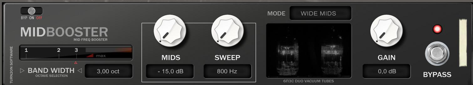
**MIDBOOSTER** is a modern parametric booster which allows adjustments to be made to the midrange frequencies of an incoming signal using parametric tuning. It can be used in your mix to add new midrange frequencies or to cut out those which aren't required.
