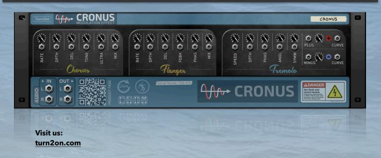
Phasing, flanging, and chorus use much of the same technology as echo and delay units. All of them are based on delay effects with a relatively small range of delay. We decided to enhance these delay-based effects with LFO modulation for the Delay effects to create special sounding effects.
