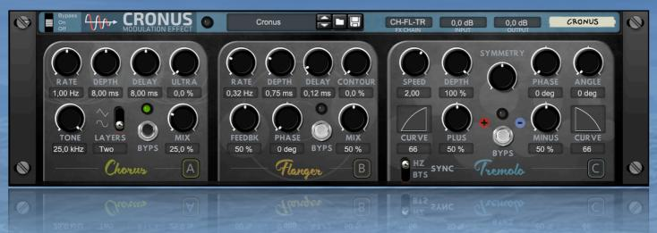
Introducing **CRONUS**, a new time-modulation effect that includes 3 effect types in one: Chorus, Flanger and Tremolo. All of these effects are time-modulated delay effects.
