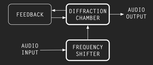
In this configuration, the input audio is sent to the frequency shifter first. The output from the frequency shifter is sent to the diffraction chamber, and from there into the feedback loop. The feedback loop routes the sound back into the diffraction chamber. The result is that the shift in pitch becomes a more prominent part of the sound.
