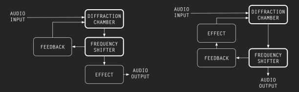
In the leftmost image above, the effect unit has been placed <u>after</u> the main feedback loop. This allows the effect unit to process the full output of the feedback loop.
