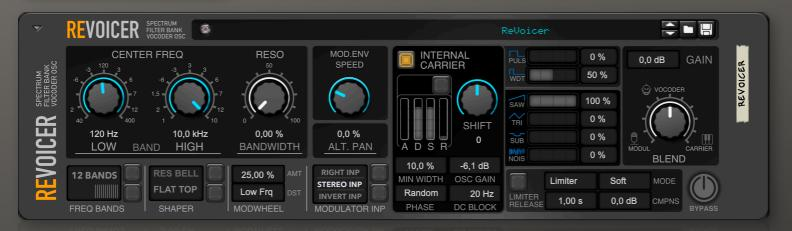
Vocoders rely on two signals being present at the same time in order to operate. These signals are the **Carrier** signal, which normally takes the form of a synth, and the **Modulator** signal, which normally takes the form of a human voice, although other instruments can work well (such as drums).
