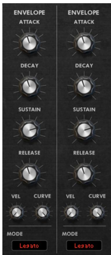
The two envelopes provide a modulation signal that typically would be used to shape filter cutoff or volume. In VK-2, the envelopes can shape anything that has a modulation input. The envelopes are typical ADSR analog-style envelopes common in many synthesizers.
