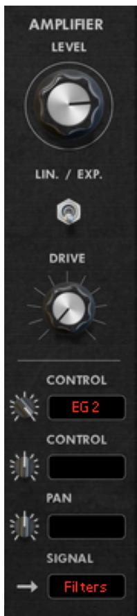
The right Amplifier section provides a voltage controlled amplifier. It is typically used after the filters in the signal path as the output stage of the synth. Note, the effects are connected just prior to the Amp section output in the signal path.
