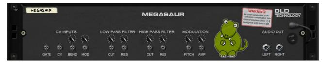
Megasaur has various CV inputs to control the sound from external oscillators and sequencers.
