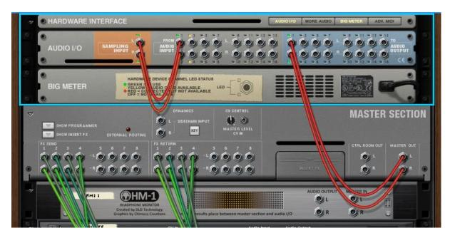
Disconnect the cable from Master Section to Audio Output 1
