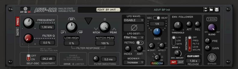
A State-Variable Filter is an active filter that uses multiple feedback techniques to produce filter responses (LowPass, BandPass and HighPass) from a <u>single filter with user selection</u>.
