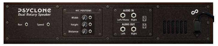
**Run** and **Speed** can be controlled via bipolar CV inputs. Remember that "Brake" is the middle state of **Speed**, so use a square/pulse wave type or direct CV values of -1 and 1 if you want to switch directly between only Slow and Fast.
