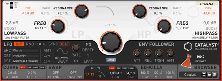
**CATALYST 2**, a new version of the hybrid multi-filter. The main function of the device is centered on the "LP/HP Morphing Filter" section. Here you can customize the LowPass and HighPass filter parameters individually, using the LP / HP filter morphing with Cutoff. The available independent settings of the LP / HP filter parameters are Resonance, Frequency, and Boost Shelf-filters.
