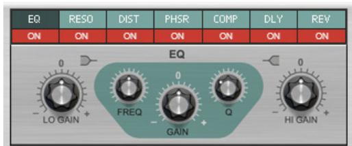
The Effects section features seven different effect modules that can be freely reordered by dragging & dropping. Most of the effect parameters are available as destinations in the Modulation Matrix, see ["Modulation Matrix"](#).
