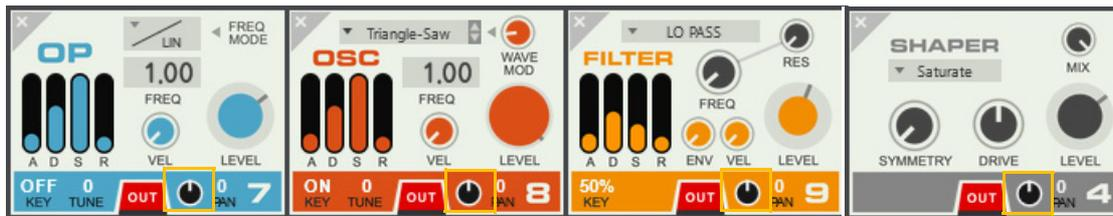
The Pan parameter is only shown and enabled if the Out button (see “Out” above) is on (red).
