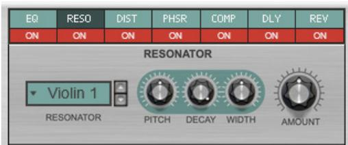
The Resonator is a convolution-based resonator/body effect with 21 built-in resonator types (impulse responses). It has a huge effect on the final sound and is great for giving a sound a certain character.
