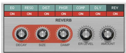
This is a stereo algorithmic reverb with control over high frequency damping and Early Reflections level. The Amount parameter works as a Send level and can be modulated in the Modulation Matrix.
