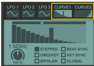
There are two separate Curve generators available for modulating selectable parameter(s) in the Modulation Matrix, see [“Modulation Matrix”](#). The Curve generators can serve as additional LFOs, semi-step sequencers or even additional envelopes.
