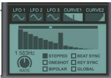
The LFO & Curves section features three separate LFOs and two separate Curve generators for parameter modulation purposes. The modulation destinations can then be freely assigned in the Modulation Matrix, see ["Modulation Matrix"](#).
