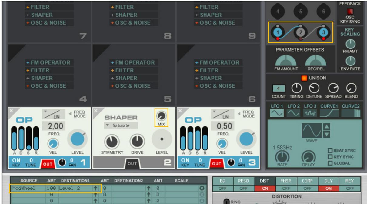
In the patch above, FM Operator 1 is frequency-modulated by FM Operator 3. FM Operator 3 is also routed directly to Out so we can hear its audio as well.
