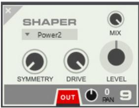
A shaper (wave shaper) distorts the incoming signal in various ways, by multiplying the input signal with a transformation function. It can distort an audio signal routed to its input, or it could change the timbre of an FM modulator, if the Shaper output is routed to the input of an FM Operator.
