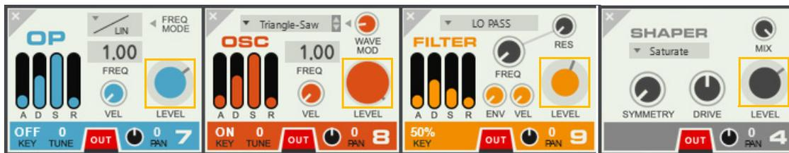
This determines the (maximum) output level from the operator. The level affects both the output volume (if the operator connects directly or indirectly to Out) and the FM amount (if it connects to the input of an FM operator) or AM amount (if it connects to the input of an Oscillator).
