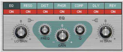
The EQ has high and low shelving bands with fixed frequencies, plus a parametric mid band.
