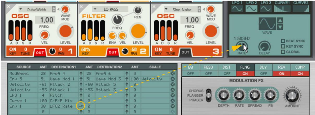
Assigning LFO 2 Rate as Destination for the Envelope of the operator in Slot 1.
