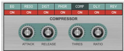
This is a stereo compressor with attack, release, threshold and ratio controls. To adjust the level after compression, use the Master Volume of Algorithm.
