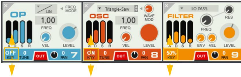
Key determines how much the Frequency (pitch) of the operator (or cutoff/center frequency of the Filter) should track the keyboard notes. If you set this to OFF, the operator frequency will be fixed (where FREQ 1.00 matches the pitch/frequency of a C3 note). Set to 50% the pitch (or filter) tracks the keyboard 0.5 semitones per note. Set to ON, the pitch (or filter) tracks the keyboard 1 semitone per note.
