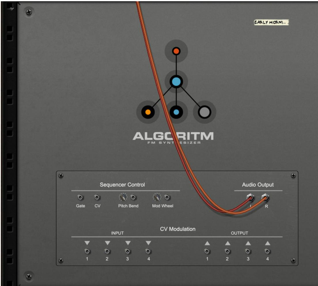
! Remember that CV connections are NOT stored in the Algorithm patches! If you want to store CV connections between devices, put them in a Combinator device and save the Combi patch.
