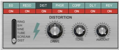
The Distortion effect offers six types of distortion with drive, tone and amount (dry/wet).
