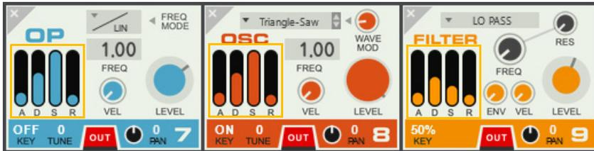
The ADSR envelope controls the output level (or cutoff/center frequency for the Filter, if the Env knob is up) over time, with the Level parameter determining the maximum output level.
