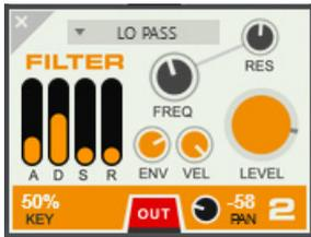
This is a state variable (SVF) resonant Lowpass/Bandpass/Highpass filter with a 12dB/octave slope. The filter is similar to the State Variable Filter in the Europa synthesizer.
