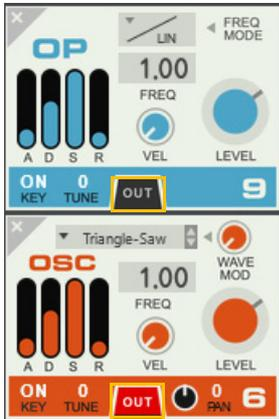
3. Click and hold the FM Operator output connector in the Routing section, drag to the input connector of the Oscillator and release the mouse button:
