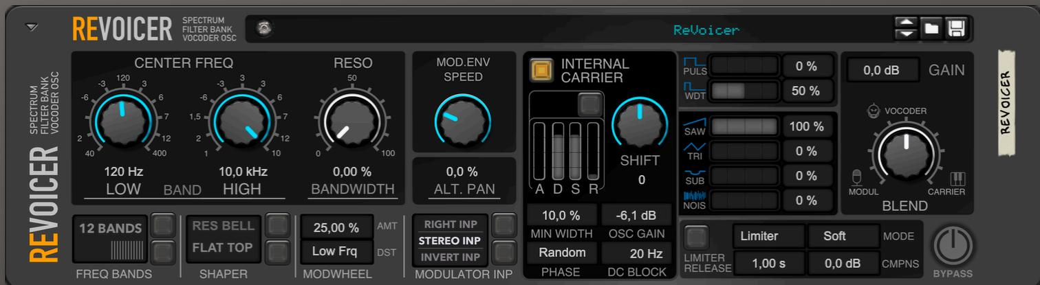
Vocoders rely on two signals being present at the same time in order to operate. These signals are the **Carrier** signal, which normally takes the form of a synth, and the **Modulator** signal, which normally takes the form of a human voice, although other instruments can work well (such as drums).
