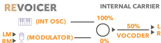
The **Classical mode** is a **Mono** Vocoder. This mode is available in **ReVoicer** when you choose Modulator source: Right Input. You can experiment with Carrier sounds with external signals by connecting your carrier signal to the Left channel. Alternatively, you can use the Internal Oscillator in ReVoicer.
