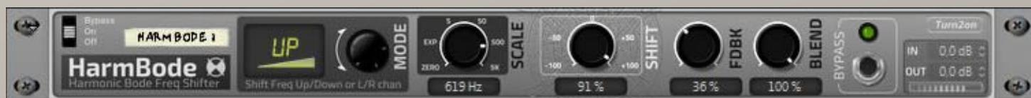
Introducing a variation of a legendary analog frequency shifter. **HARMBODE** shifts the spectrum of a signal by a fixed amount. BODE (TM) Shifter is not a pitch-shifter, but allows you to shift inharmonics in Hz. Sometimes it can sound like a ring modulator effect, but with HARMBODE it is possible to get an upshifted and downshifted signal. With some settings you can hear the effect known as "Barberpole flanger" as well as a 90 degree phase shifter.
