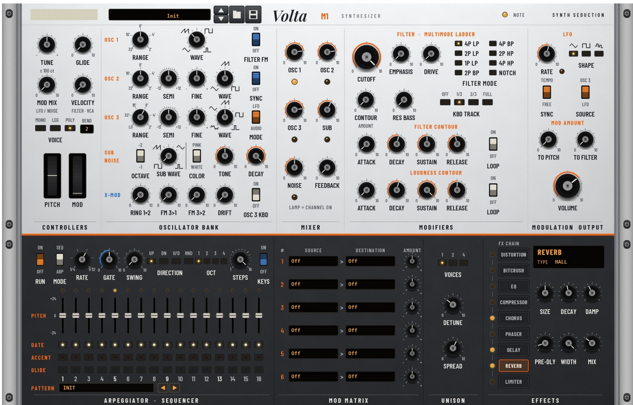
Volta M1 front panel (7U). The upper section is the synthesizer; the lower section holds the sequencer, matrix, unison and effects.
